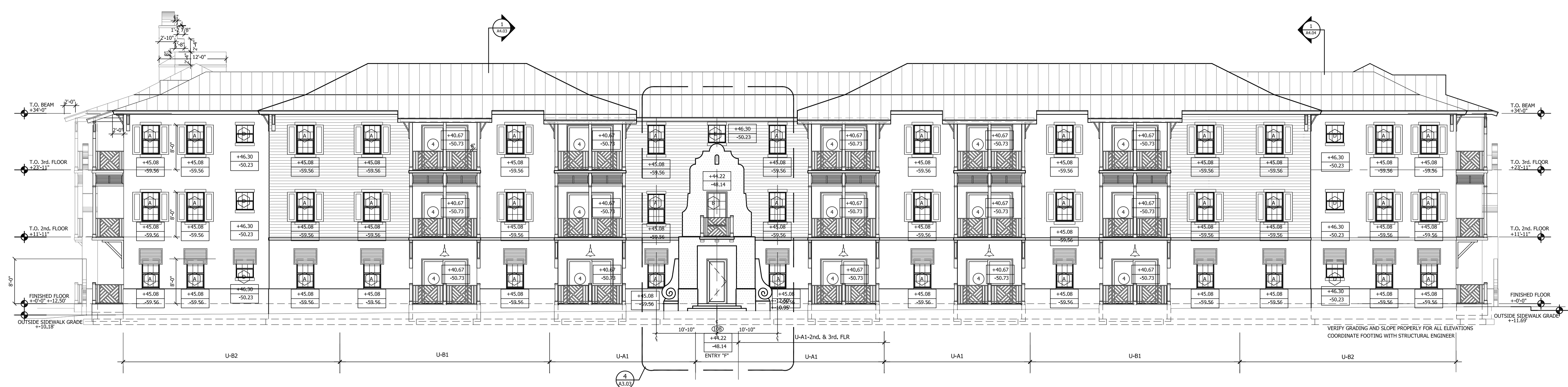
4 WEST 2nd. STREET ELEVATION "D" BLDG ELEV. SCALE: 3/32"=1'-0"
